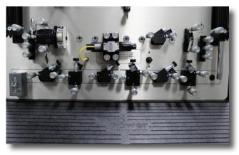
Component storage slots on front of trainer allow quick and easy access to most commonly used components
