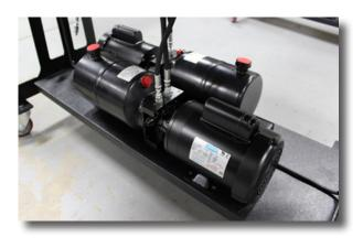
Power unit and self-contained reservoir is located at the bottom of the trainer.
